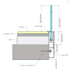
Installation on terrace with pedestal-mounted slabs
